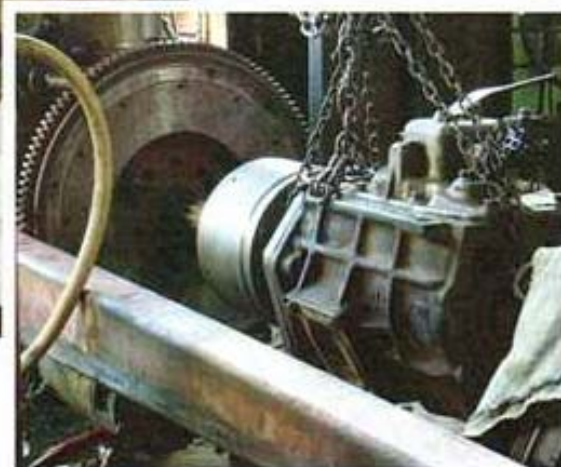
Moving the gearbox into position to see how everything would line up.
