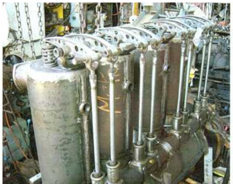
Camshafts, pushrods and rockers in place. Water jackets have now been fabricated around the CAT sleeves. The engine is starting to take shape.
