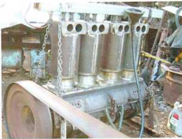
Engine being belt driven to run in the rings, sleeves and bearings. Note the oil feed (funnel) used to supply the main bearings with oil. The valves were also held open during the operation.
