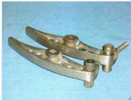
Stages involved in making the rockers which were modelled on some early aero engine rockers Nev had seen and admired.
