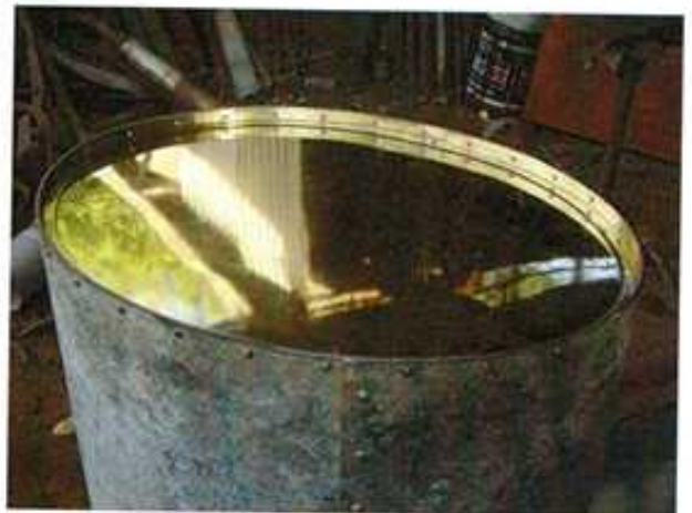
Nev fabricated an authentic looking fuel tank by rolling a galvanized skin and then he made brass ends which were polished and riveted into place. The tank was later painted and a hand-pump was used to pressurize the tank and supply fuel to the carburettor.
