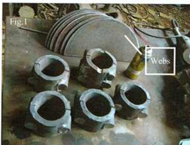
3"x1" flat steel were pressed to form semi circles. These had bolting flanges welded on, which had holes bored so they could be bolted together in pairs to form the main bearings.
