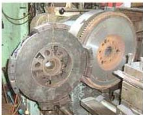
Facing the flywheel and preparing the heavy duty clutch.
