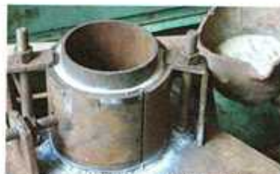
The molten babbitt after being poured into the mould.
