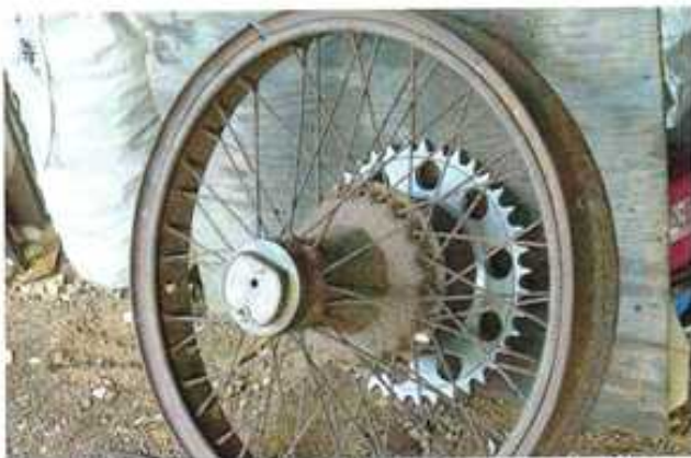
One of the 24" Budd wire wheels with a finished sprocket fitted. Nev later sandblasted the wheels and painted them before fitting new tyres.
