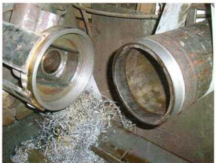
The stages of fabricating the heads with inlet and exhaust ports.
