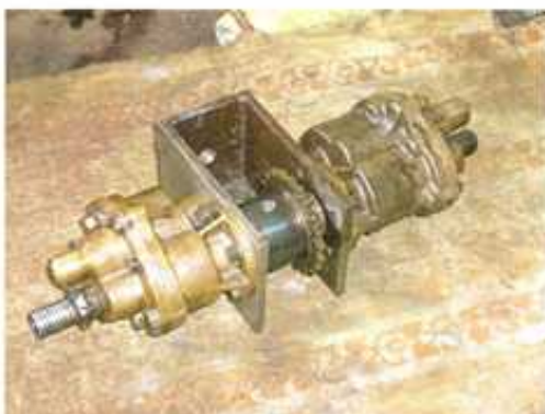
The two oil pumps coupled together.
