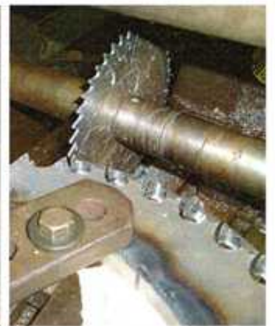
The rear sprockets in various stages of manufacture - small guide holes were drilled at first, then larger holes were drilled and then the apex of the teeth were cut out with a milling cutter. Some hand finishing was required to tidy up the sprockets.
