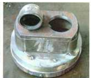
The stages of fabricating the heads with inlet and exhaust ports.
