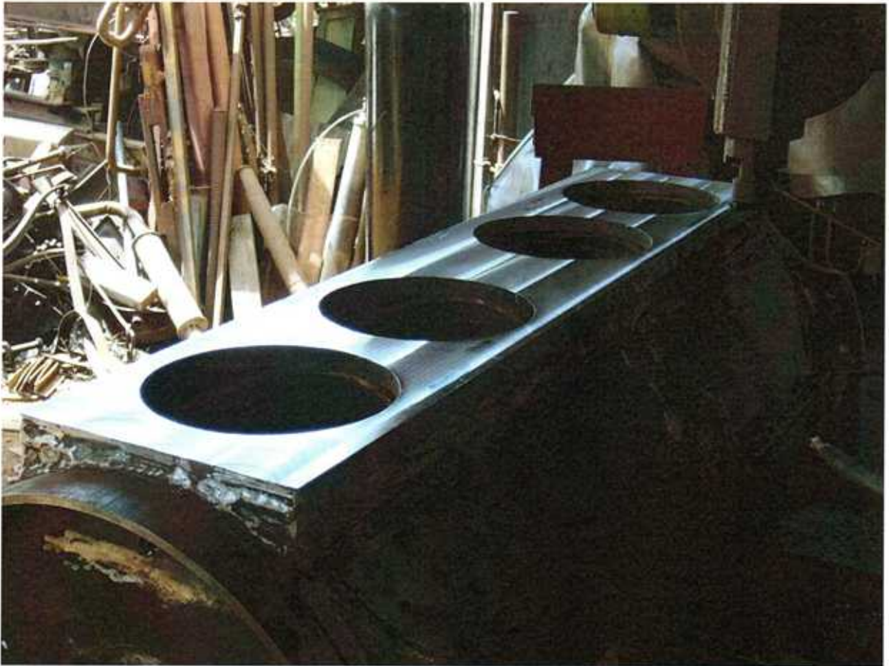
Cincinnati milling machine completing the facing of the cylinder mounting platform.
