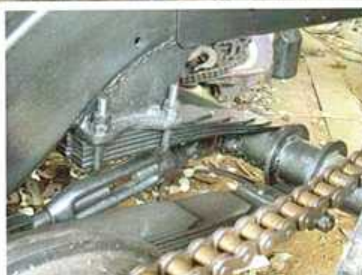
(Above) The Ford diff fitted to the Buick chassis and the rear axle and chain in place. Note the original brake drum fitted to the diff which would provide some stopping power.
