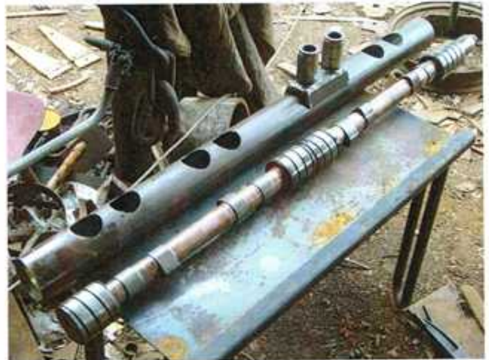
(Top left) A cylinder sleeve on the lathe so piston rings can be cut to the required size. (Top right) The cam shaft and its housing beginning to take shape. (Bottom left) Closing the ring gap before clamping between two plates for final machining.
