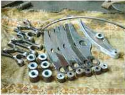
Stages involved in making the rockers which were modelled on some early aero engine rockers Nev had seen and admired.
