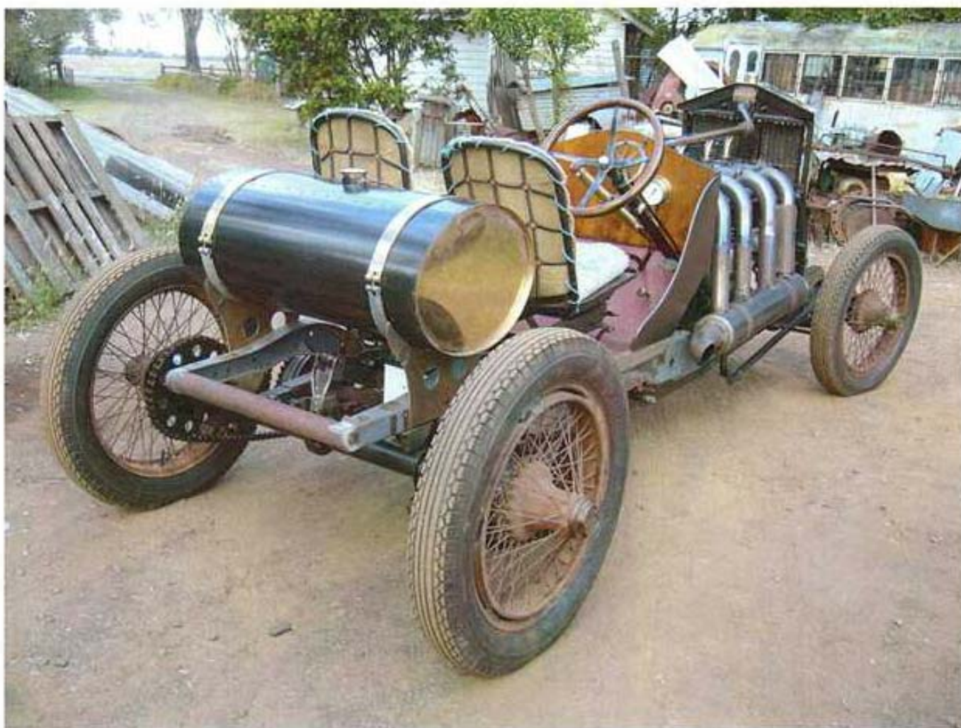
SOG emerges from the shed on its wheels for the first time. Note that the right-hand rear wheel has the 24" rim welded onto the 23" wheel. A 24" wheel was fitted later.
