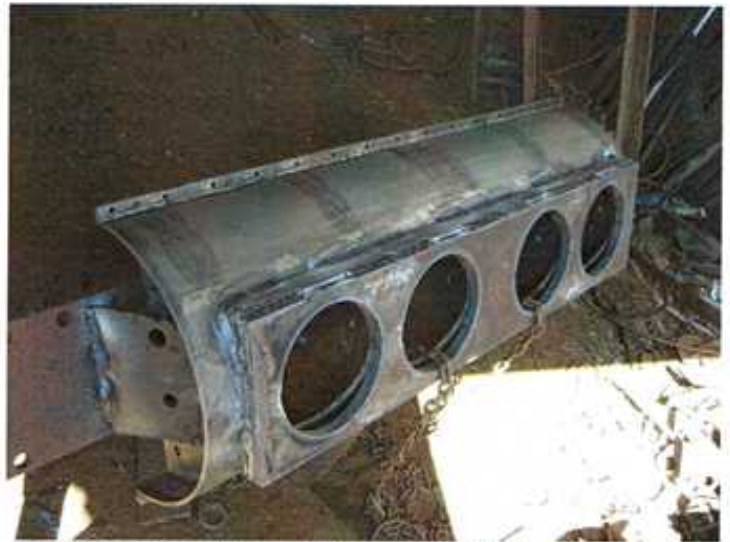
Cylinder mounting platform completed and ready to be machined.
