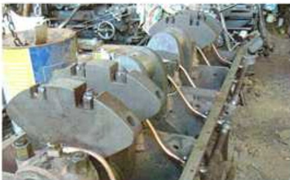
(Above) Five pipes feed oil to the main bearings from a larger external oil line.
