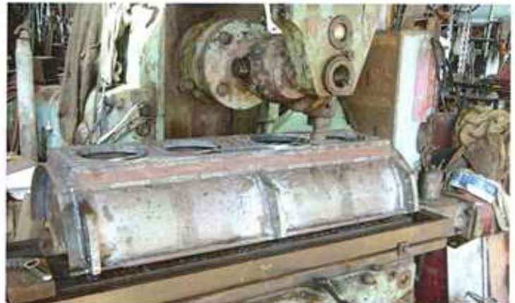
A Cincinnati milling machine was used to face the cylinder mounting platform and bore the holes to their correct size to accommodate the CAT D9 sleeves.
