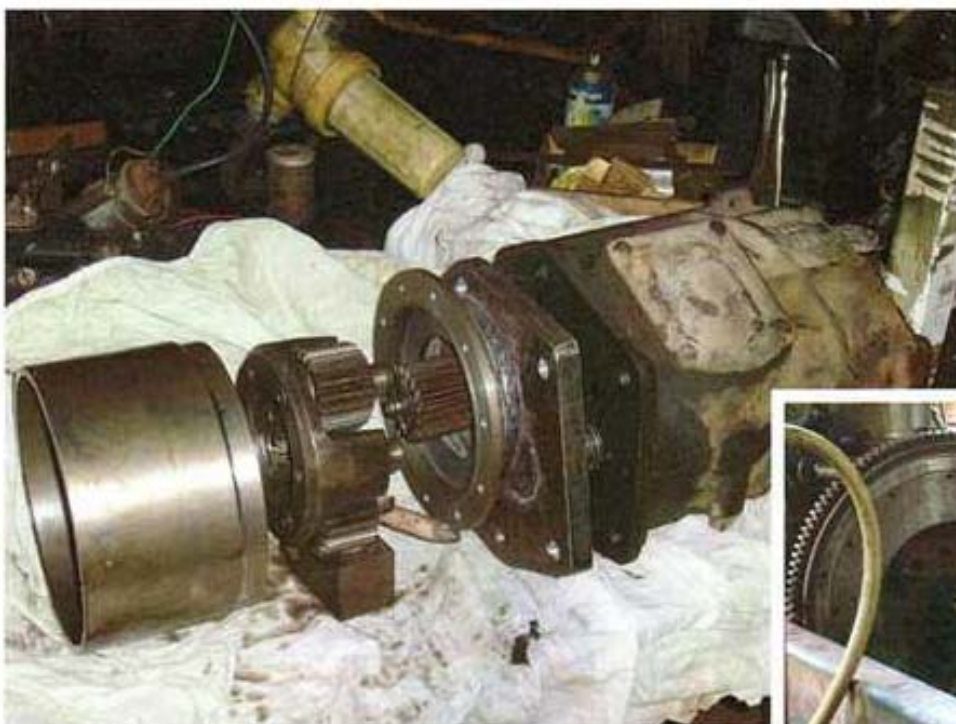
Assembling the Albion reduction drive and fitting it to the five speed gearbox. In its new role, the reduction hub multiplies the engine RPM by 3 to achieve the desired overall gearing.
