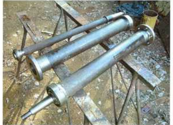
The two piece rear axle has bolting flanges in the middle.
