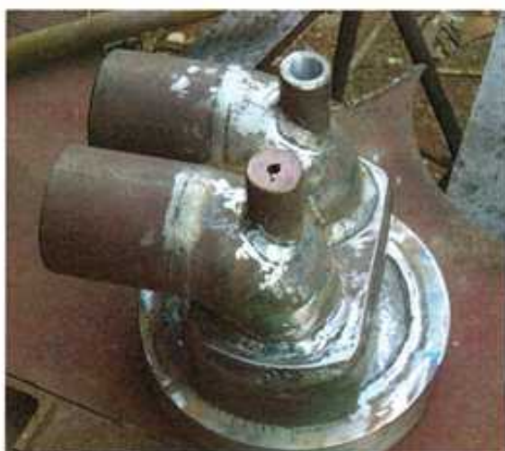
(Above) Five pipes feed oil to the main bearings from a larger external oil line.
