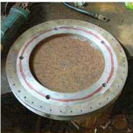
The rear sprockets in various stages of manufacture - small guide holes were drilled at first, then larger holes were drilled and then the apex of the teeth were cut out with a milling cutter. Some hand finishing was required to tidy up the sprockets.
