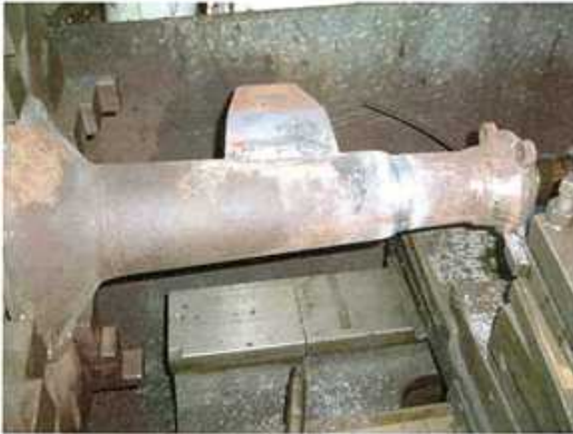
The 37 Ford diff housing after it has been shortened and welded.
