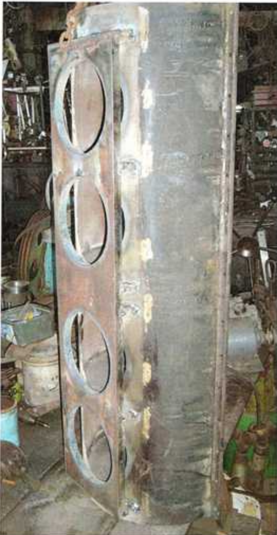
Cylinder mounting platform taking shape.
