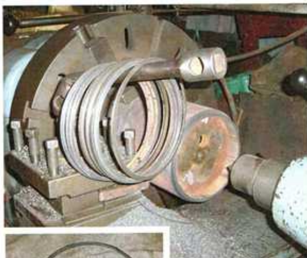
(Top left) A cylinder sleeve on the lathe so piston rings can be cut to the required size. (Top right) The cam shaft and its housing beginning to take shape. (Bottom left) Closing the ring gap before clamping between two plates for final machining.
