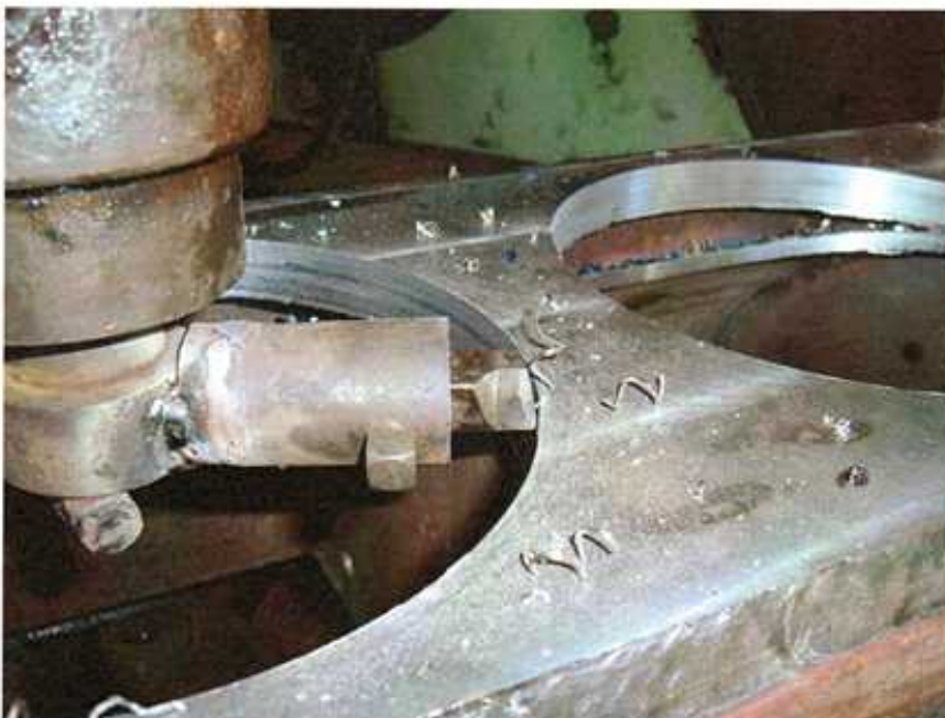
Close-up of the Cincinnati milling machine boring the holes to their correct size to accommodate the CAT D9 cylinder sleeves.
