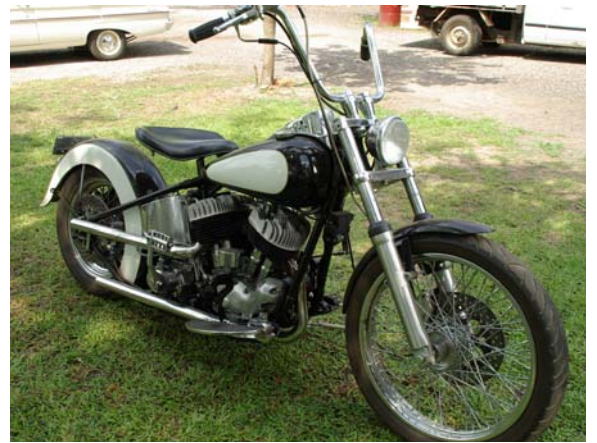
Yet another sidevalve Harley. 1938 1200 UL. The engine and frame are original but has modern wheels and brakes.
