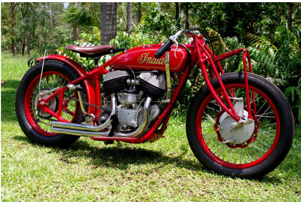
1924 Scout with 1200 Chief motor. The combination is commonly known as a "Chout" This bike pulls 13.3 secs on the drag strip at Hidden Valley. And that's with the foot clutch and hand gear change too. All these bikes have the original Indian setup of the throttle on the left hand side of the handlebars. This is one of the bikes in the old photo and this, Dick says, is his favourite bike.
