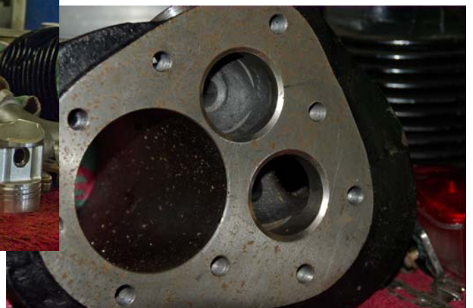
Modified barrel . Note the uppermost valve is as big as it can possibly be
