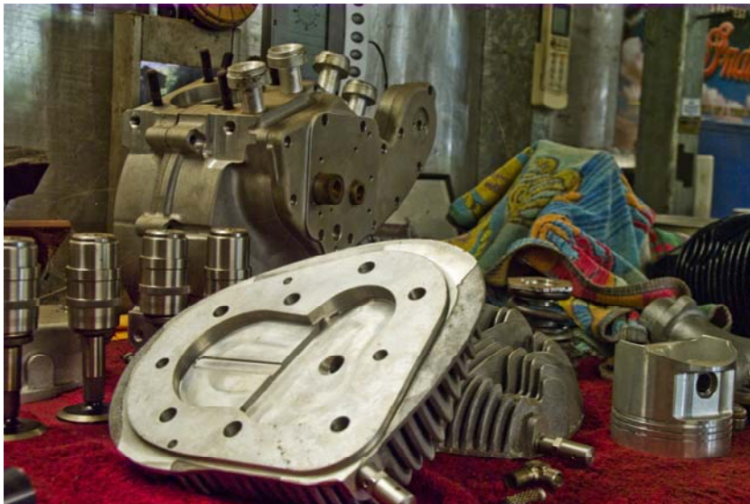
Below: Another high performance Indian motor in the process of being built. Note the recess for the piston in the head. The piston comes within 30 thou of it.
