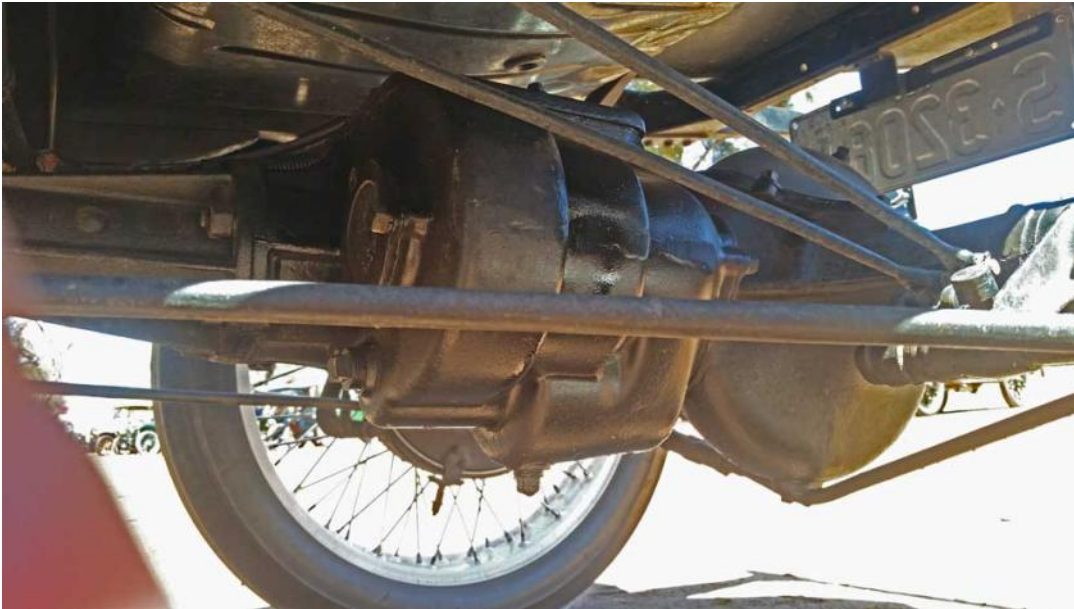
Two views of the gearbox mounted at the diff end of the torque tube which encloses the tailshaft, which spins at engine speed.
