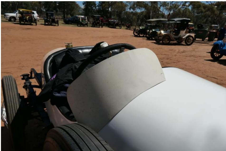
No nothing for the passenger/navigator/ engineer, but the driver does get a wind deflec- tor. Large diameter steering wheel functions as power steering.
