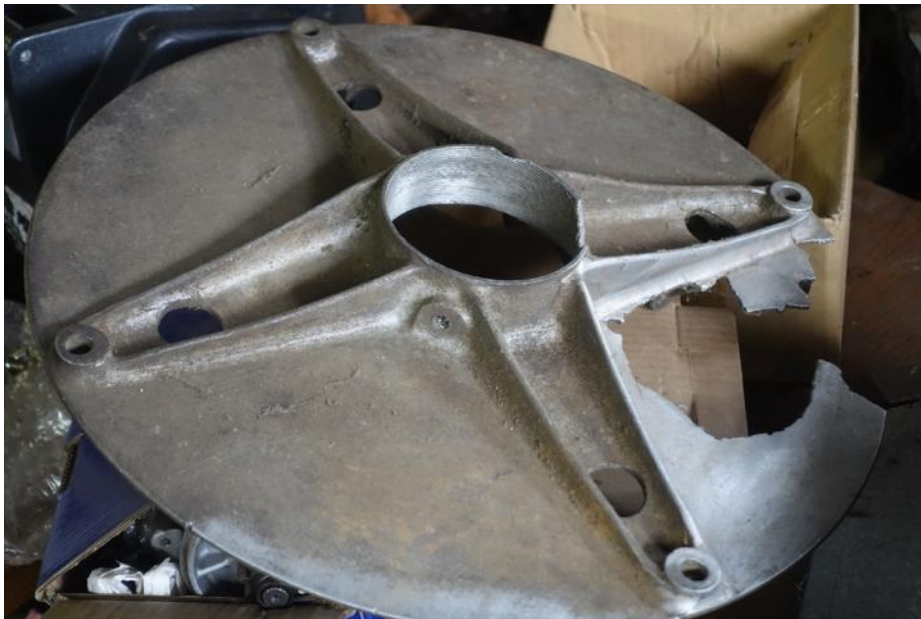
Part of the clutch pressure plate. They had to cast a new one. This car has a fairly conventional disc type clutch. One step away from conventional though is the clutch plate is steel. And it works well and doesn't slip.
