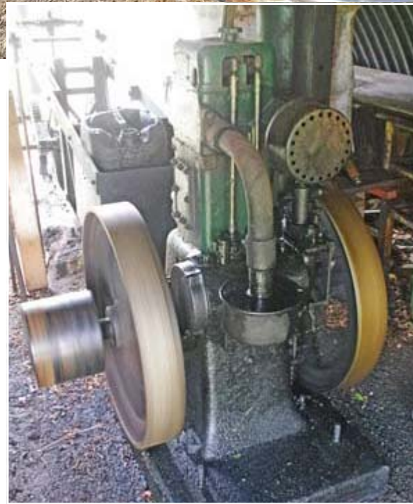
The water in this household comes from a bore. To get the water from the depths is a vintage Kaesler pump jack made nearby in Hahndorf, driven by the venerable Lister single cylinder engine. Starts and runs a treat!
