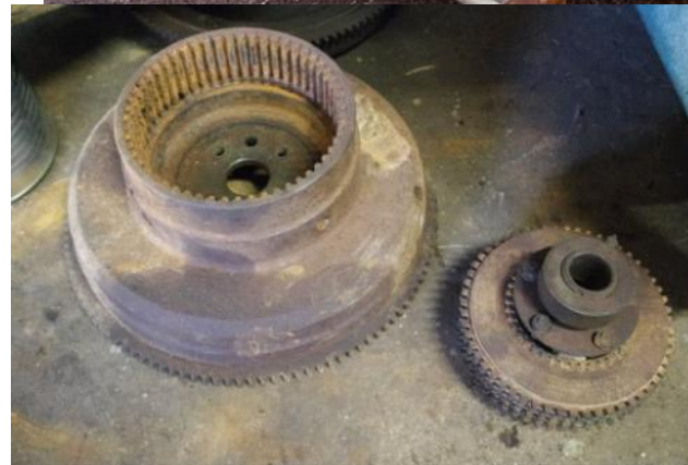
The multiplate clutch and flywheel.
