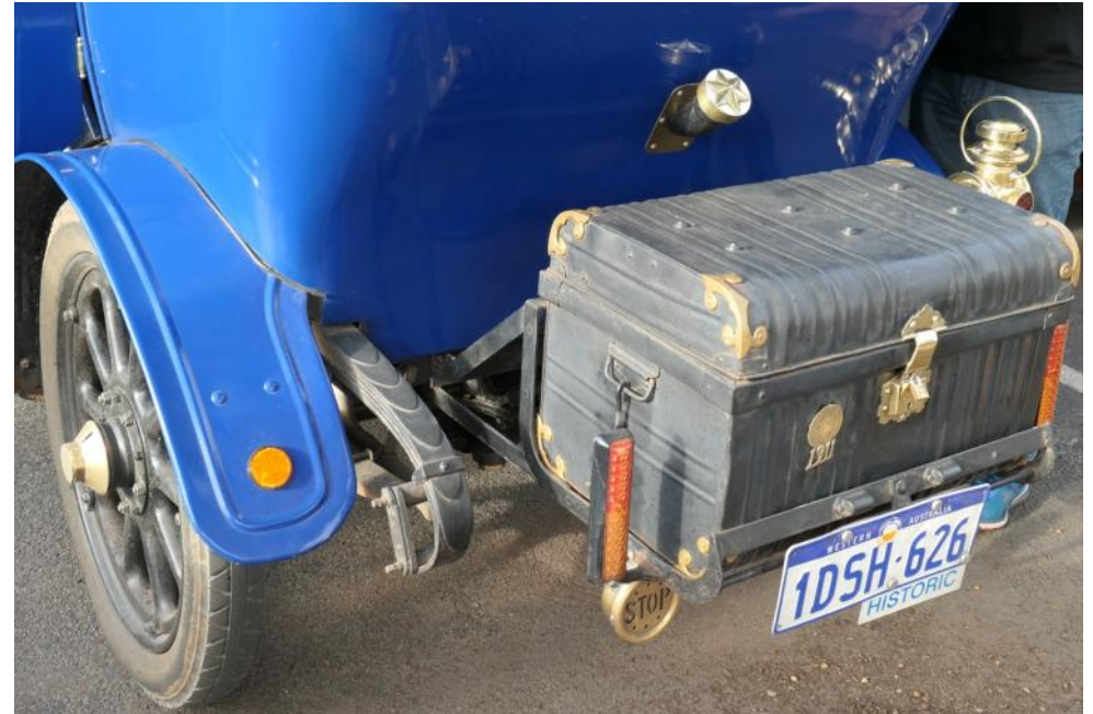
The wheels are actually aluminium, cast from the original wheels.
