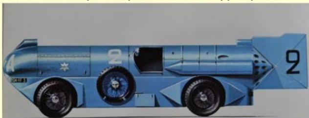
It was a sight to behold and looking much like a streamlined military machine, it had a large cylindrical body and a vast tailfin, and M Stapp revealed it had a trio of 29litre Bristol Jupiter radial aero engines, from which he had removed the pistons and converted them to what he described as 'internal combustion turbines.'
