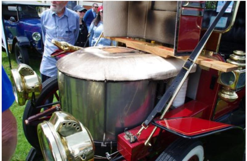
*Under the bonnet you don't find an engine, Instead there is the boiler. Runs at up to 600psi.*
