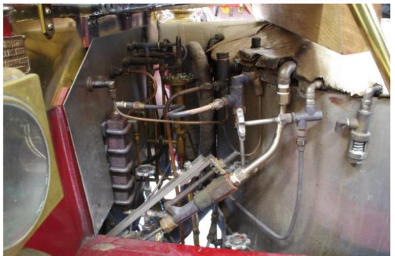
*Behind the boiler is a mass of pipes and valves. To the right of the photo is the blow off valve if it all gets out of hand.*
