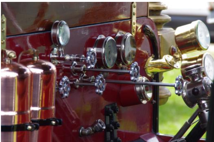
Left: Clear uncluttered dash panel. Note the instrument light attached to the steering column facing forward. You still need to see those knobs and gauges after dark.
