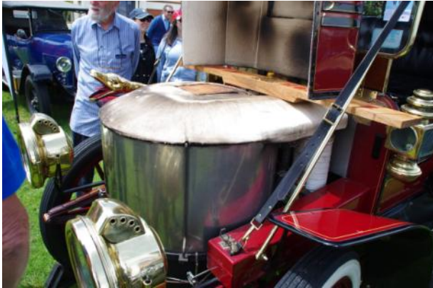
Under the bonnet you might expect an engine. Not with this car, you get a boiler.
