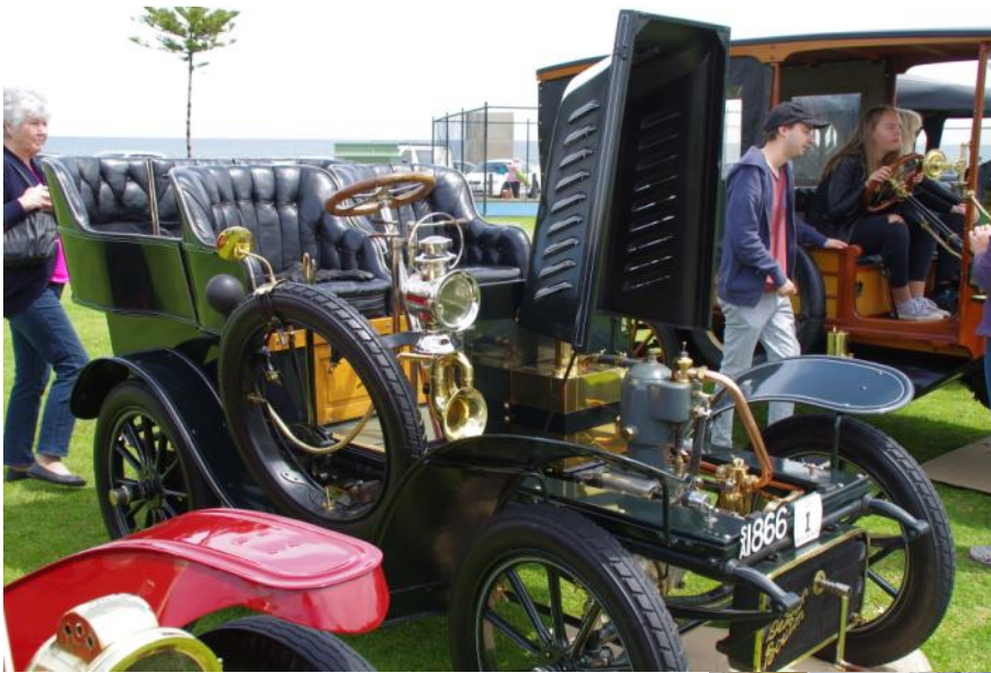
Under the bonnet you might expect an engine. Not with this car, you get a boiler.
