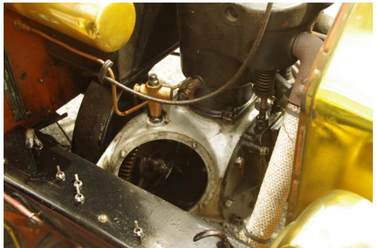
The 1 litre single powerplant. The cover is off to reveal the counterbalance gear. Elsewhere in the engine compartment is a Selden plate. This indicates Brush paid Selden a royalty to sell a motor car as Selden had patented the idea of motorised transport (see stuff on the net,)
