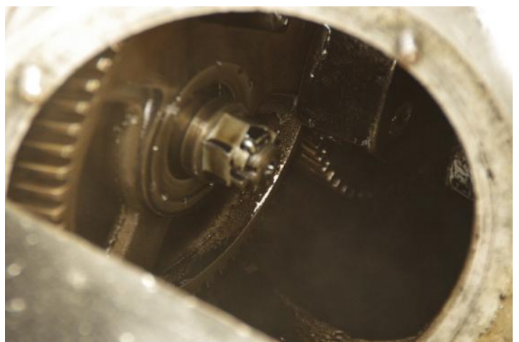
The 1 litre single powerplant. The cover is off to reveal the counterbalance gear. Elsewhere in the engine compartment is a Selden plate. This indicates Brush paid Selden a royalty to sell a motor car as Selden had patented the idea of motorised transport (see stuff on the net,)
