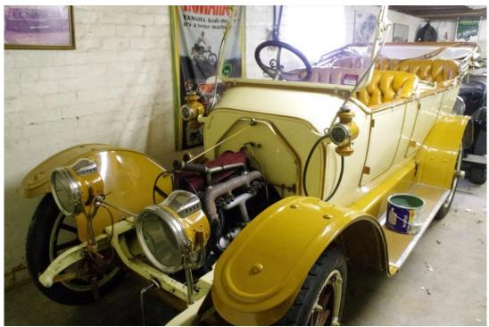
The Buick currently has its radiator removed due to the crankshaft pulley repairs.
