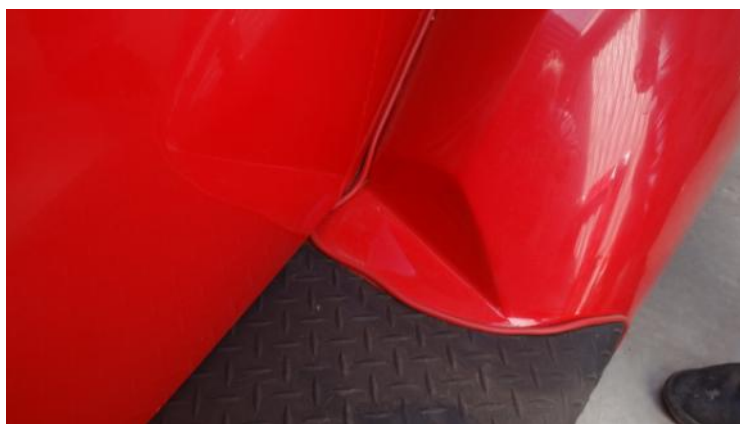
Cut outs in the front guards for the door openings are a legacy of mixing 2 different models
