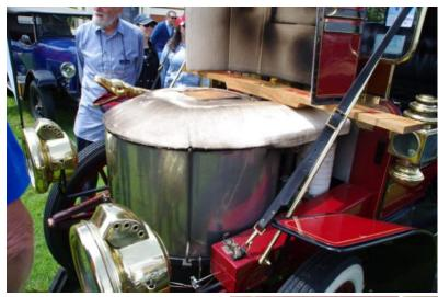
Under the bonnet you don't find an engine, Instead there is the boiler. Runs at up to 600psi.
