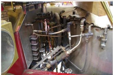
Behind the boiler is a mass of pipes and valves. To the right of the photo is the blow off valve if it all gets out of hand.
