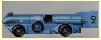
It was a sight to behold and looking much like a streamlined military machine, it had a large cylindrical body and a vast tailfin, and M Stapp revealed it had a trio of 29litre Bristol Jupiter radial aero engines, from which he had removed the pistons and converted them to what he described as 'internal combustion turbines.'
