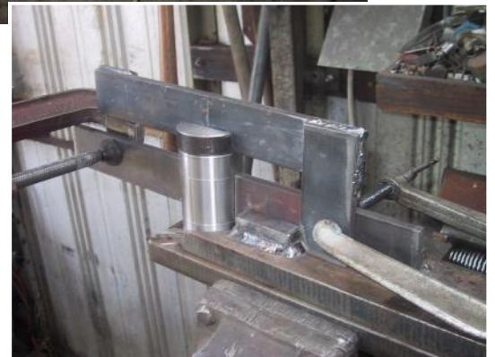
The jig for welding the straight spokes to the hub
